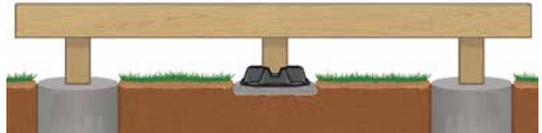
Use BLOCK along with concrete footings on Hybrid-Profile decks
