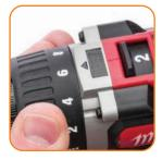
If your drill has a drill and clutch mode, set it to clutch mode. Turn down torque to the lowest setting. Increase as necessary.
