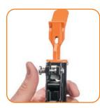
Insert the Edge nose piece. It will lock into place.
