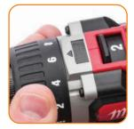
If your drill has a drill and clutch mode, set it to clutch mode. Turn down torque to the lowest setting. Increase as necessary to fully drive screw. **Do not overdrive.**
