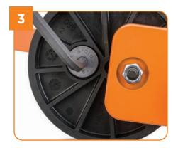
**TIGHTEN** Use supplied hex key to securely tighten the screw.
