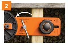
**POSITION** Place LEVER on the joist and tighten the joist cam with the pivot pin
