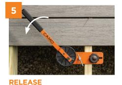
Release pressure by moving the handle away from the deck board.
