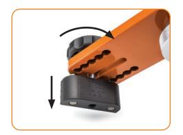
Loosen joist knob until the stop block disengages.
