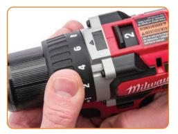
If your drill has a drill and clutch mode, set it to clutch mode. Turn down torque to the lowest setting. Increase as necessary to fully drive screw.
