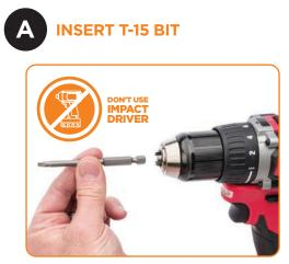
Insert the T-15 driver bit into your drill. Do not use an impact driver.
