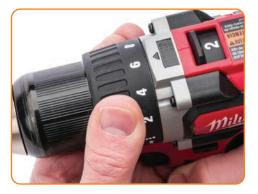
If your drill has a drill and clutch mode, set it to clutch mode. Turn down torque to the lowest setting. Increase as necessary.
